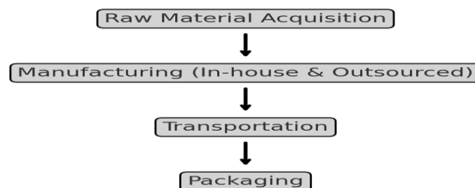
System Boundary Diagram (Cradle-to-Gate)
