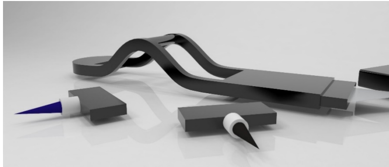
Figure 10: A Mouse for Computer Work for Disabled People Using a Foot
